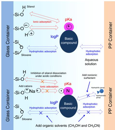
Fig. 1 Mechanism of Adsorption to Vials and Methods for Inhibiting Adsorption
