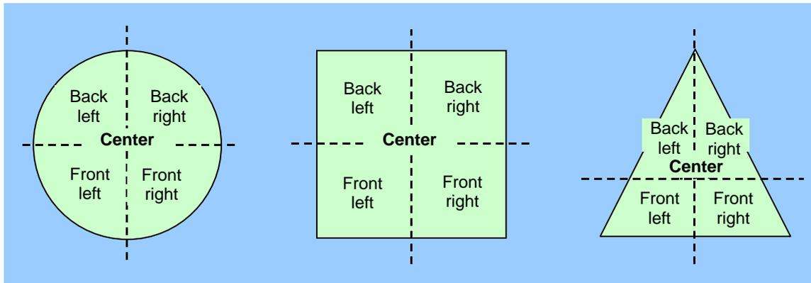
6-2-3. Linearity (Inspection is performed for both the small and large ranges in the case of dual-range electronic balances.)
