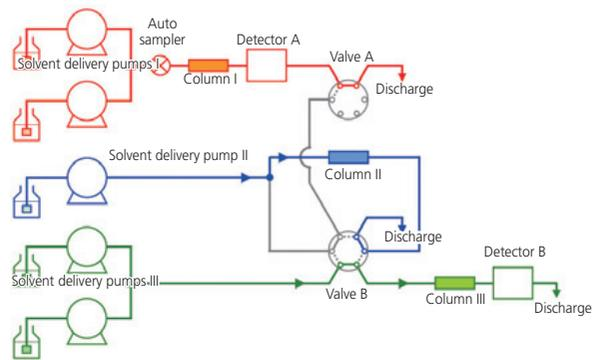
Fig. 3 Flow Line Diagram for Co-Sense for Impurities System
