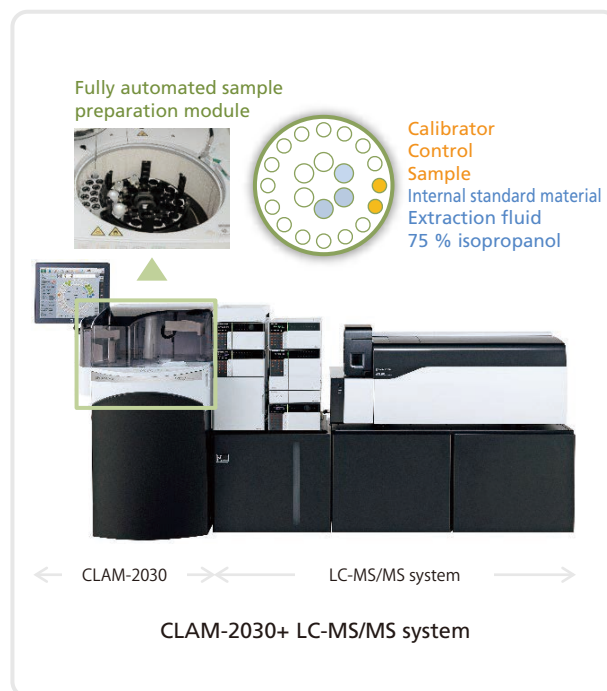
Fig. 6 Sample preparation for voriconazole using CLAM-2030
