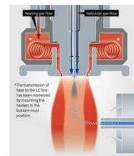
Figure 3. Heated ESI probe
