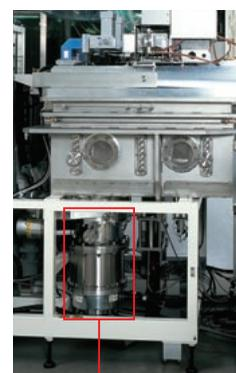
Turbomolecular pump for flat-panel production
