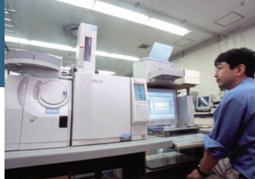
Shimadzu's GCMS, being used to effectively monitor water quality at a water purification plant in Japan
