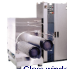
Glass winder (used to wind glass fibers)
