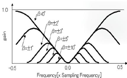
**Fig. 3** Differences in Cut-Off Frequency According to X-Ray Tube Swing Angle
