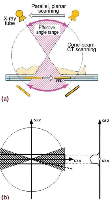
**Fig. 2** (a) Image Reconstruction by FBP Method and (b) Band Limitation
