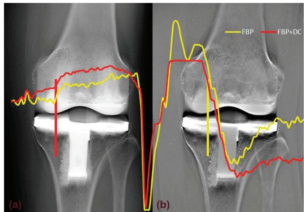
**Fig. 8** Image and Profile Curve Before and After Adding DC Component
