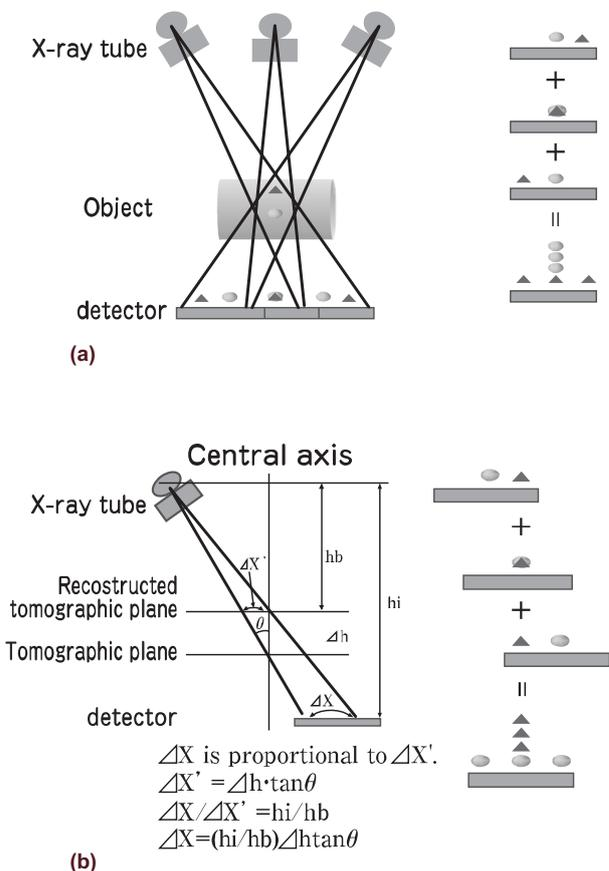
**Fig. 1** (a) Principle of Tomography and (b) Shift-and-Add Method
