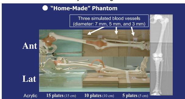
Fig. 8 “Home-Made” Phantom Used for Visual Evaluation
