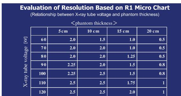
Fig. 7 Results of Evaluation of Relationship Between Subject Thickness and X-Ray Tube Voltage Based on R1 Micro Chart
