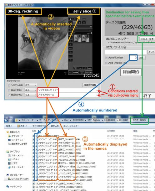
Fig. 5 Windows for Fluoroscopy Image Recording System
