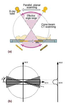
Fig. 2 (a) Image Reconstruction by FBP Method and (b) Band Limitation
