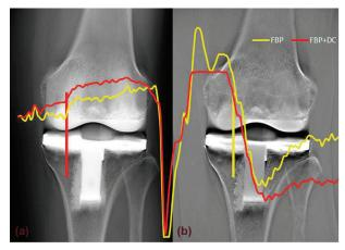
Fig. 8 Image and Profile Curve Before and After Adding DC Component (a) After (b) Before
