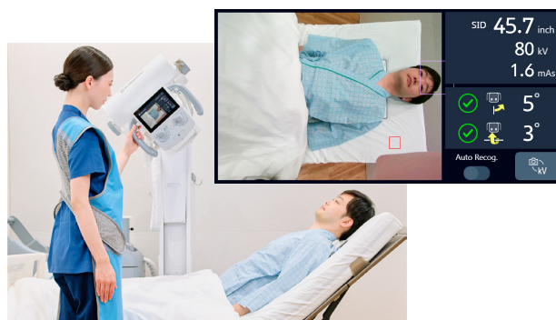
Fig. 7 Measurement of distance and angle using the 3D camera
