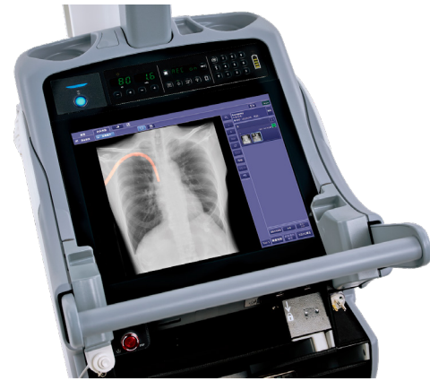
Fig. 9 Tube and Catheter Enhancement Image Processing (Smart Tube™)
