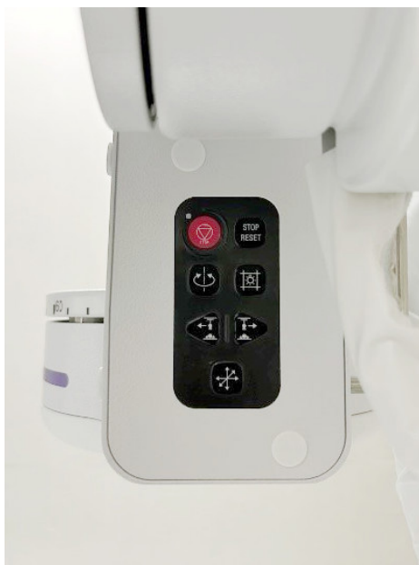
Fig. 7 Rear Switches on Column Section
