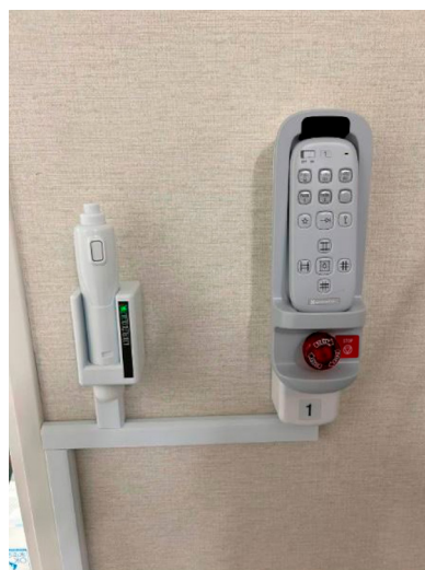
Fig. 5 Left: Wireless Hand Switch (Bluetooth) Right: Remote Control for Auto Positioning (Infrared)
