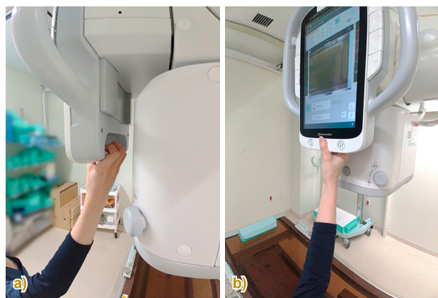
Fig. 6 a) Recess on the back of the X-ray tube support operation panel. b) Front All-Free switch.
