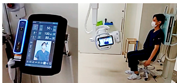
Fig. 1 Display on the X-ray control console (left image) and display on the X-ray tube support (right image).
