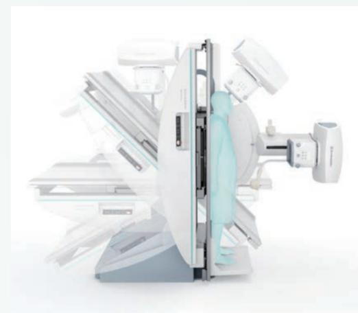
The table tilting functions are designed with soft-start and soft-stop actions to minimize patient anxiety caused by sudden movements. In the standing position, the edge of the tabletop is 5 cm from the floor. The minimum step height is 10 cm from the floor, making it easier for patients to step up or down from the table. A sensor at the table edge automatically stops tilting actions if part of the foot is being pinched.
