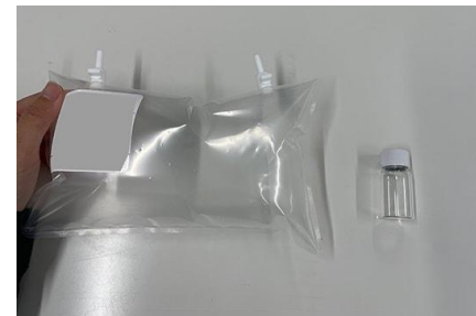
Gas-bag sampling combined with compact vial extraction
