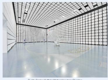
Quality Center 10-Meter Method Anechoic Chamber
