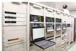
NICT Japan Standard Time System (Cesium Atomic Clock)
