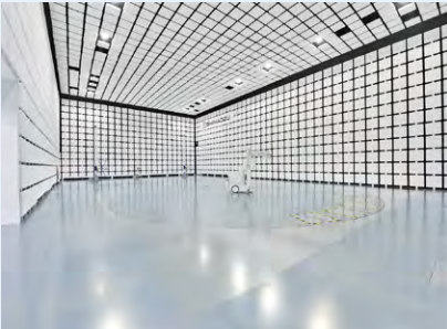
The Quality Center is equipped with a 10-meter anechoic chamber for EMC testing.
