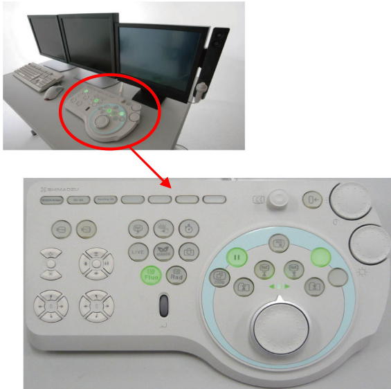
Fig. 13 Controller for Control Room: IVR Shuttle
