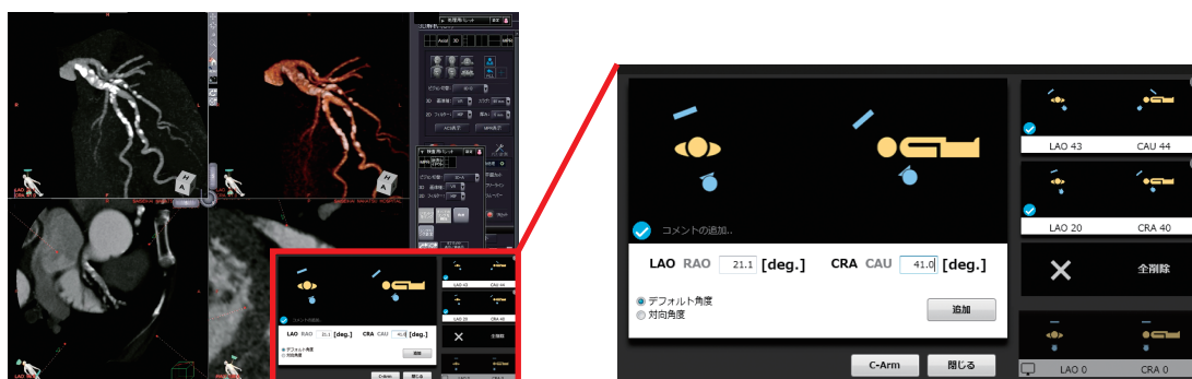
Working angle determined from CT images of the LAD and D1 bifurcation lesion, and angle transmitted to the C-arm.
