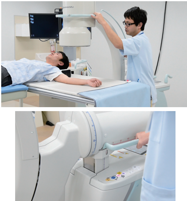
Fig.3 C-Arm can be moved quickly by manually moving it vertically or horizontally
