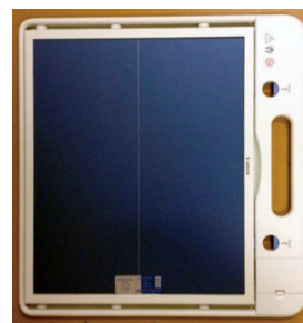
Fig. 8 Dedicated Handle Unit It includes a carrying handle, which makes the FPD heavy and makes determining the center of the grid difficult.
