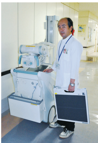
Fig. 3 New Thin, Light, Easy-to-Use Large-Field-of-View FPD
