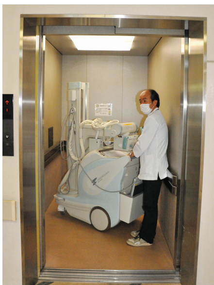
Fig. 5 Maneuvering the Unit in an Elevator Power-assist function permits maneuvering in a confined space.
