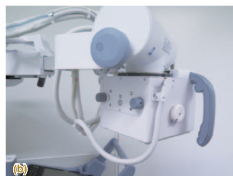
Fig.6 Front (a) and Back (b) of Collimator Exposure field lamp buttons and exposure field aperture knobs are provided on both sides.
