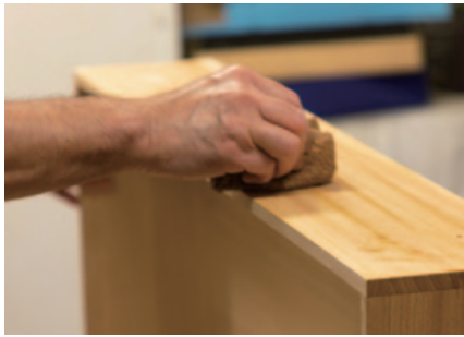
The boxes are coated with tonoko to finish. The majority of tonoko is created in Kyoto's Yamashina district.
