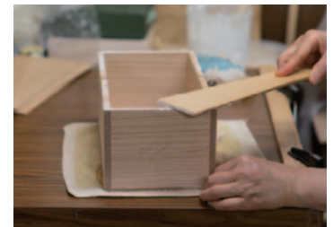
The adhesive is uniformly tapped onto the box using a special spatula. Once the adhesive has been applied, it is kept in place by a thick rubber band to dry.
