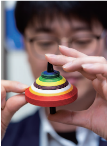
Checking whether the thread is horizontally wrapped at a uniform width. If any threads stick out, it is cut off with scissors.
