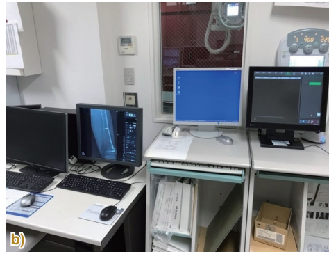
Fig.4 Remote Controllers for Automatic Positioning for Radiography in Standing and Supine Positions Controller for Standing Position (Left) • SID150: Lateral view of thoracic vertebrae, lateral view of lumbar vertebrae, etc. • SID180: Chest, cervical vertebrae, etc. • SID200: Auto-stitching radiography • Park: X-ray tube position when not in use Controller for Supine Position (Right) • Home: Anterior view of lumbar vertebrae, etc. • AXIAL: Axial position of patella, etc. • Park: X-Ray tube position when not in use
