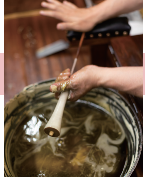
The final uvaro layer is applied using the kigake method. Applying too much wax will mean the candle won't have a clean white finish. After, the top and bottom are cut to shape.
