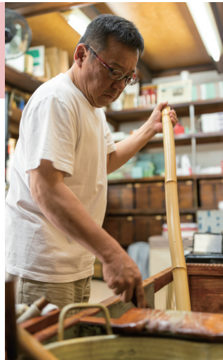
Air is kneaded into the melted wax with a thick bamboo pole to generate the perfect consistency.
