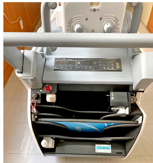
Fig.6 Stores One 17 × 17 Inch FPD, One 11 × 14 or 10 × 12 Inch FPD, and One Grid
