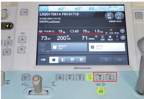
Fig.5 Use of the Key Customization Function to Change the Pulsed Fluoroscopy Rate
