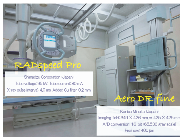
Fig.2 Appearance and X-ray conditions of the system with Dynamic Radiography ability
