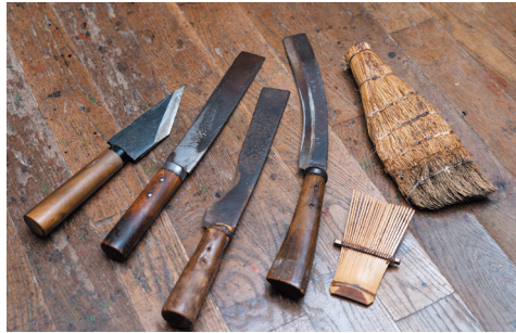
The two knives in the middle are hegi-bocho , while the two tools on the right are for applying the washi . The kaki-take , which resembles a Japanese tea whisk, is handmade and helps to ensure the glue reaches every corner.
