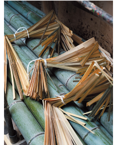
The bamboo strips are seared with a burner and bent into a U-shape. These strips are then used to create the yotsume-ami pattern.
