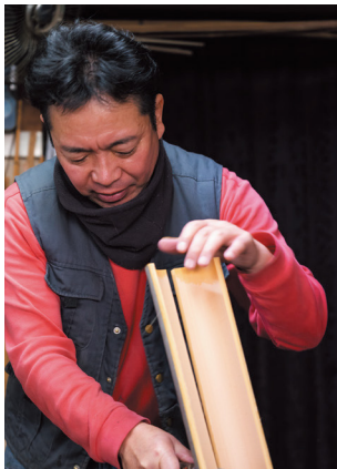
The bamboo is vigorously cut into rough sections before being cut again into sheets.
