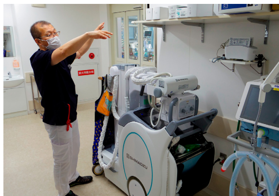
Thanks to the collapsible column, the system can even be stored under shelving.
