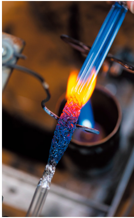
Creating the body for the Miyabi model. The blue body is held in the right hand while rotating it in a fixed direction to apply the pattern. The wave-like pattern on the thick part is made by lightly pushing on the rod.
