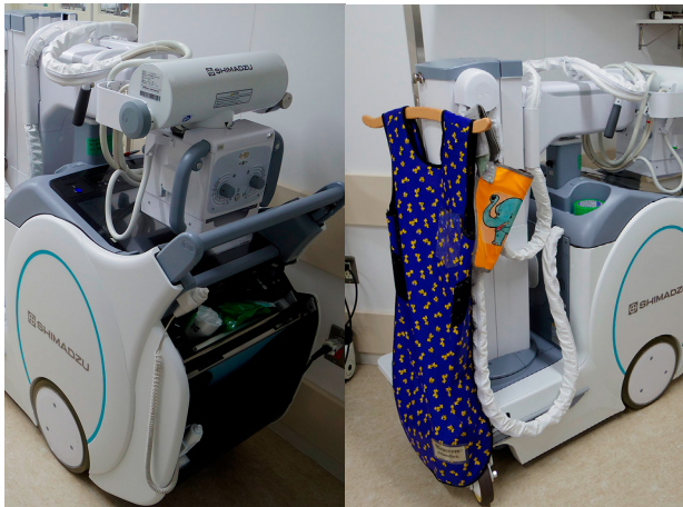
During hospital rounds, plastic bags and cleaning wipes for infection control are stored in the rear storage box of the MX8 (left). A protective apron is also carried on a hanger from the hook on the support column.
