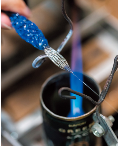
Work on the nib requires the most precision. Too much oxygen can cause the flame to become too strong and destroy the nib.
