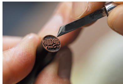
The final carving. Carving the face at an angle from the edge increases toughness and flexibility and makes the seal more durable.
