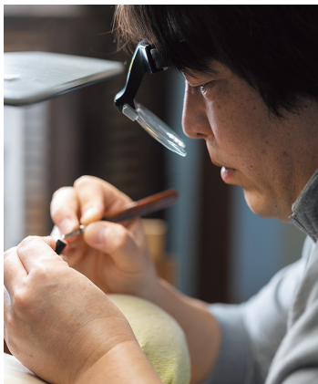
After the rough carving, the seal is removed from the holder and the craftsman switches to the finishing knife.
