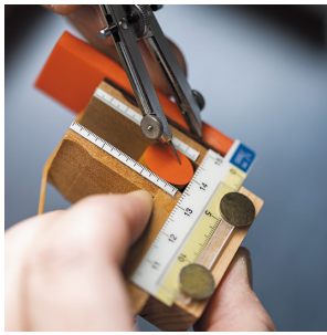
A handmade tool that holds the seal material, locates the center, and allows the craftsman to draw a grid without damaging the face.
