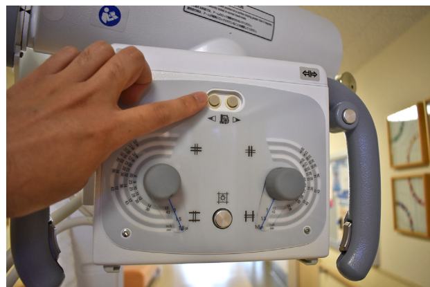
Fig.4 “Inch-Mover” Buttons. Incremental control over cart position from the collimator.
