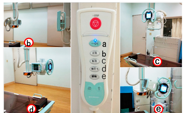
Fig.9 Auto-Positioning Remote Control a) Linked to a preset position in the generator program b) Standing SID 180 cm c) Supine d) Lateral (side view) e) Patella axial view (retract position)
