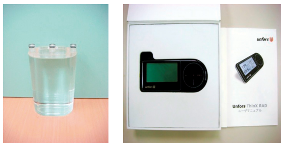
Fig. 12 Chest / Abdominal Water Phantom and Dosimeter
