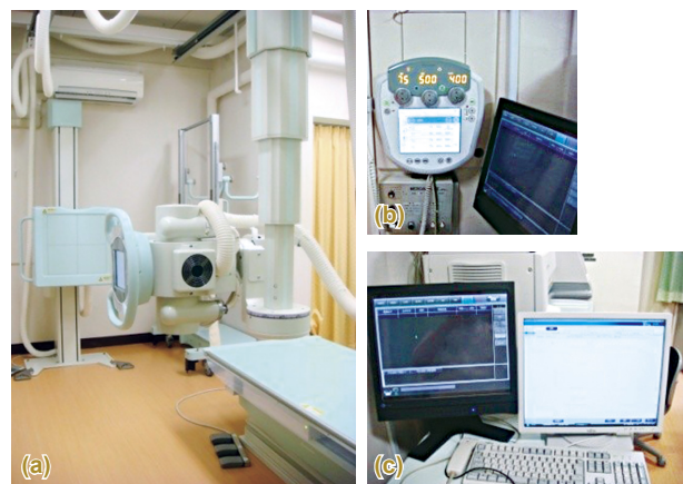
Fig. 3 (a) Appearance of RADspeed safire; (b) Operation Panel; (c) RIS Console
